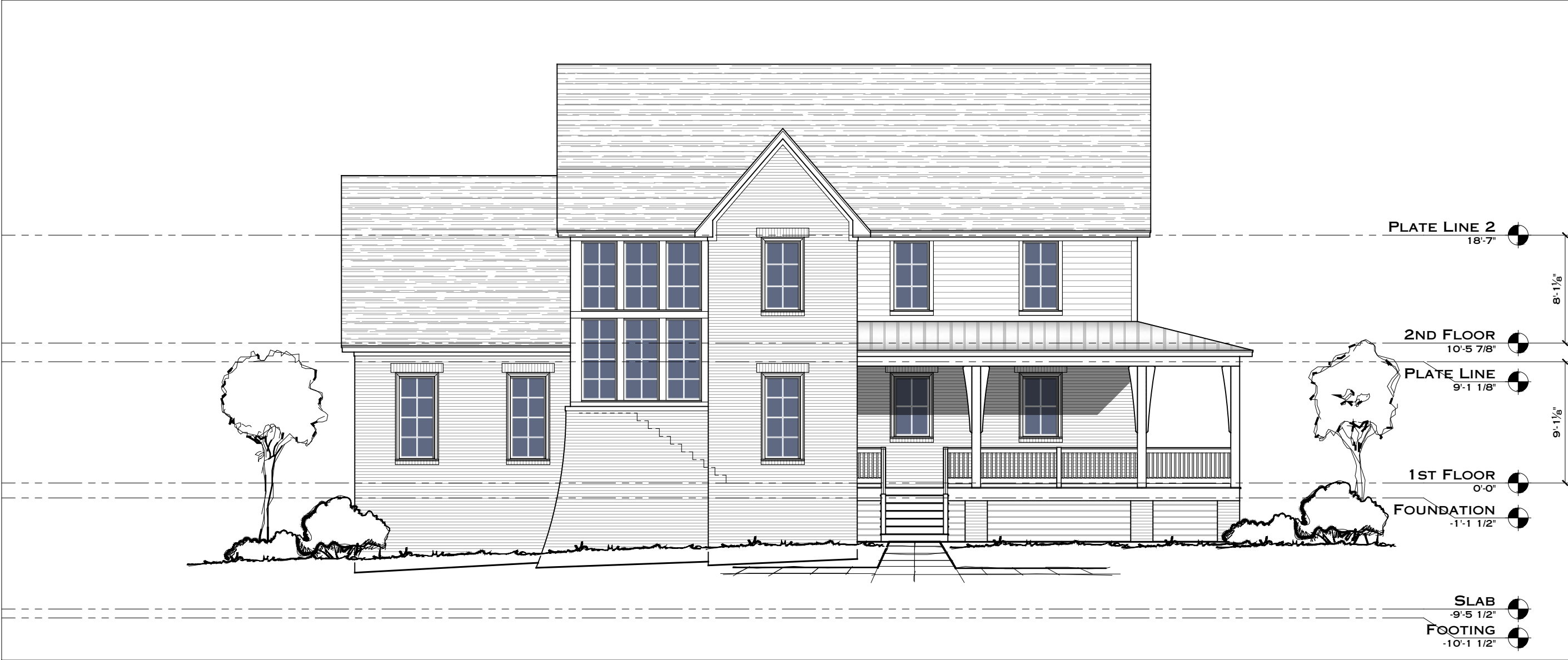
1 A3.1 Front Elevation 1/8" = 1'-0" 0 4'-0" 8'-0" 16'-0" 24'-0"
